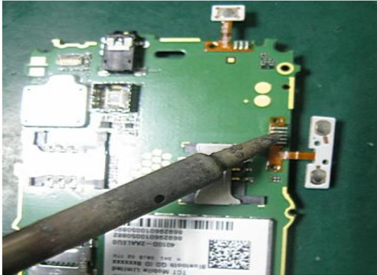
Step 9: Remove power key FPC and volume keypad FPC by using soldering iron (Temperature: Lead-free technology  $330^{\circ}\text{C}\pm 10^{\circ}\text{C}$ , time: 2~3 seconds).
