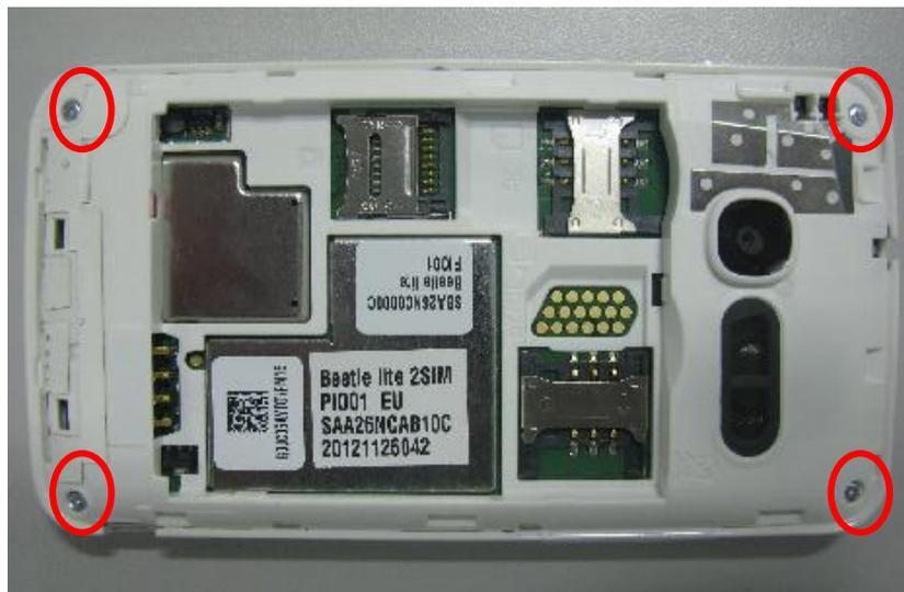
Step 3: Pry the furnished frame up by plastic flake. Then separate the furnished frame from furnished front casing.
